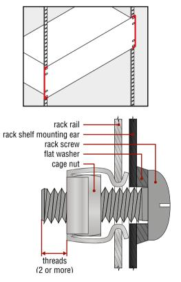
**ATTENTION!** Fix the frame to the rack rail by applying all mounting holes. Choose properly sized screws for mounting. Keep minimum two threads left after the nut screw.
