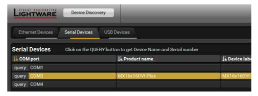
**ATTENTION!** When the device is connected via the local RS-232 port, make sure that LW protocol (#1) is set on the serial port. The protocol settings are available by the front panel buttons, see the Control Protocols section.
