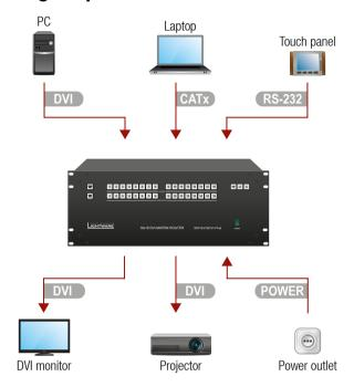
Connect the desired sources to the **DVI input ports**.
