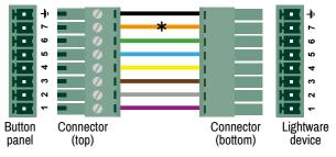
1 The cable between the button panel and the GPIO port was tested by 50 m, AWG23 cable type. For longer distance, please contact Lightware.
