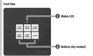
• The labels of the buttons are just for illustration since the button caps are empty by default. The user can insert the desired label from the attached sheet.
