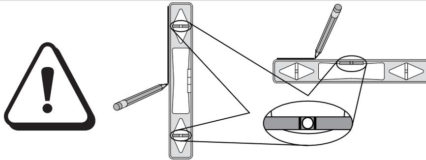
All of the lines that you draw to install the SB800ix2/SB800ix2-SMP must be straight and level on a plumb wall. You must install the unit straight, level and plumb for it to operate properly.
