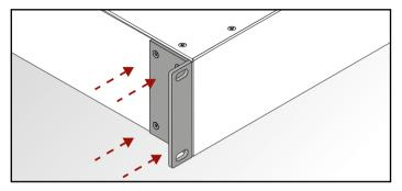
ATTENTION! M4x10 size is the longest allowed screw for fixing the ears to the housing. A longer screw may touch internal parts.
