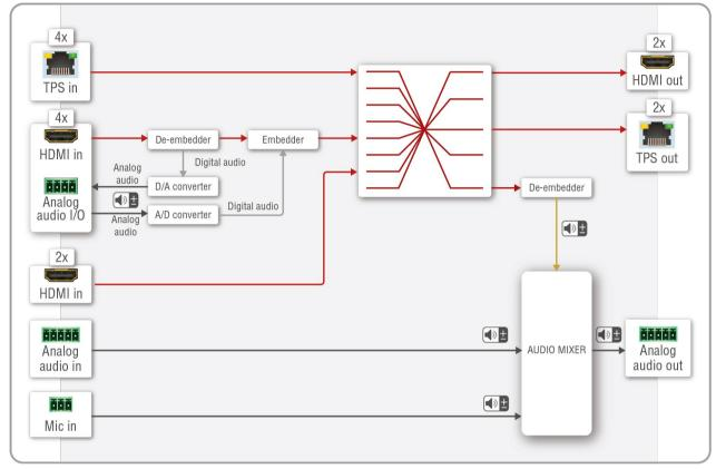
5.3.3. Port Diagram of MMX8x8-HDMI-4K-A and MMX8x8-HDMI-4K-A-USB20
