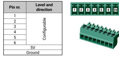
GPIO connector and plug pin assignments
