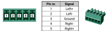
Analog audio connector and plug pin assignments
