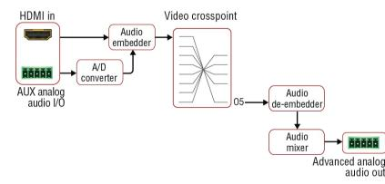
Crosspoint state: AUX analog audio I/O belongs to the HDMI port beside. To transmit the audio signal, set the appropriate video input to 05. For more details about the crosspoint switching, see Crosspoint Operations
