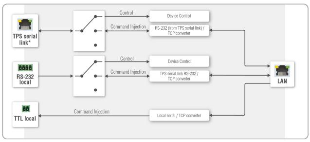
The block diagram of the Serial interface
