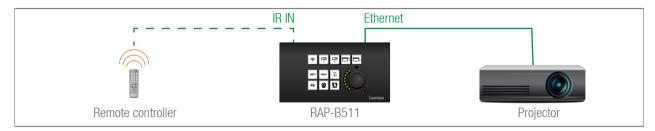
The projector can be powered on via the RAP-B511 by using the remote controller with the following way:
