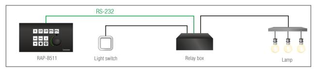
At first, configure the recognizer for the serial communication, after that, configure the Button1.
