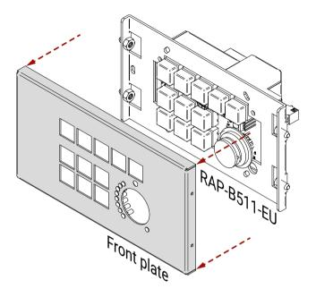
Step 2. Place two screws (marked with red color) OR four screws (marked with yellow color) in the holes.
