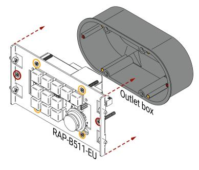
Step 4. Fasten the front side of the device to the **Outlet box** by fitting all the screws. Step 5. Place back the Front plate to the Button panel.
