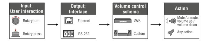
INFO: Customizing the rotary functions is possible with Lightware Device Contoller software (the details can be found in Configurations of the Rotary section) or with LW3 protocol commands (for more details see Volume Control Configuration section).
