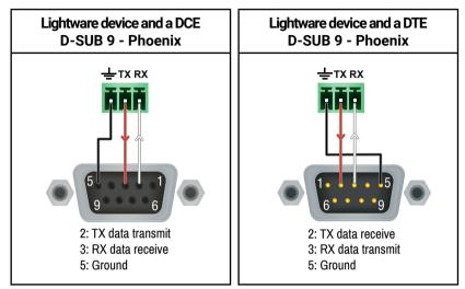
INFO: The RAP-B511 series works as a DCE unit according to its pin-out.
