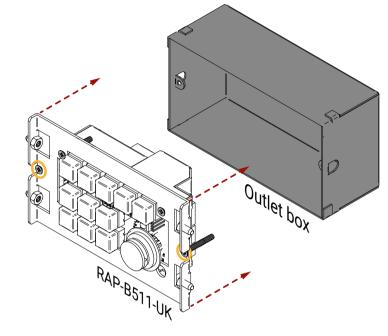
Step 4. Fasten the front side of the device to the **Outlet box** by fitting all the screws. Step 5. Place back the Front plate to the RAP-B511-UK
