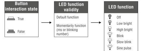
LED function settings has to be done with Software Control - Lightware Device Controller software (in UI Config Menu section) or with LW3 protocol commands (for more details see Button LED Configuration section).
