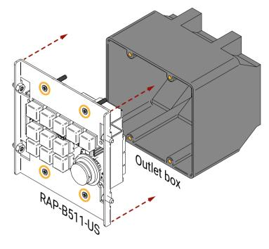
Step 4. Fasten the front side of the device to the **Outlet box** by fitting all the screws. Step 5. Place back the Front plate to the RAP-B511-US
